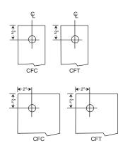
8200 **Push Plate** 8300 Pull Plate, Prep for Pull (less pull)
