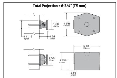
The Sentronic® SEM 7800 Series are heavy duty, electrically controlled door holding magnets. Magnets are fail safe and hold until the current is interrupted. A manual door closer is used to control and close the door. A choice of floor, recessed wall, or surface mounted wall magnets are available.
