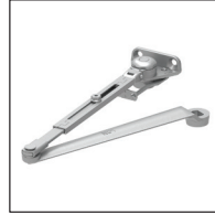
4010-3049FL Fusible link arm ▪ Handed ▪ Releases hold-open function when exposed to temperatures above 165° F. 1/8" (3 mm) maximum reveal ▪ Optional ▪ NOTE: Check local codes before specifying FL arms. NOT A life safety product!
